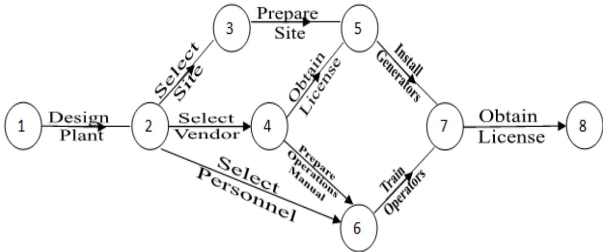
Network diagram for power plant construction
